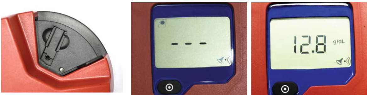
Figure 5: Cuvette holder in loading position
